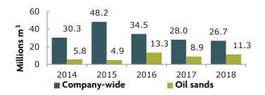
Flaring is a controlled burning of natural gas. In 2018, we had more unplanned flaring events and higher flared volumes overall at our oil sands operations compared with 2017. To better manage flaring and venting, we have a fuel, flare and vent management program aimed at improving the quality of measurement and reporting of flaring data. See our emissions data.
