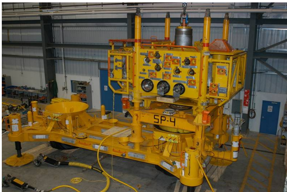
TGB with PGB and Subsea Tree at Cameron – St. John's
